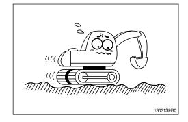
When working on soft ground, place mats or wood boards on the ground to prevent the machine sinking.
